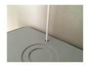
If mounting inside a metal can, the antenna must extend outside the enclosure to ensure RF communication
