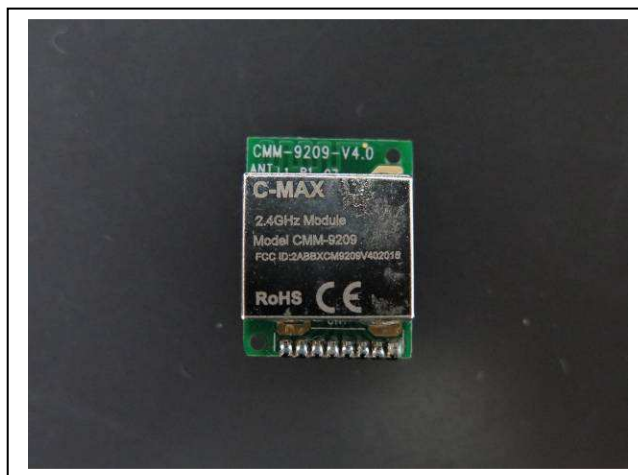
ID Label 1 (with pin header)
