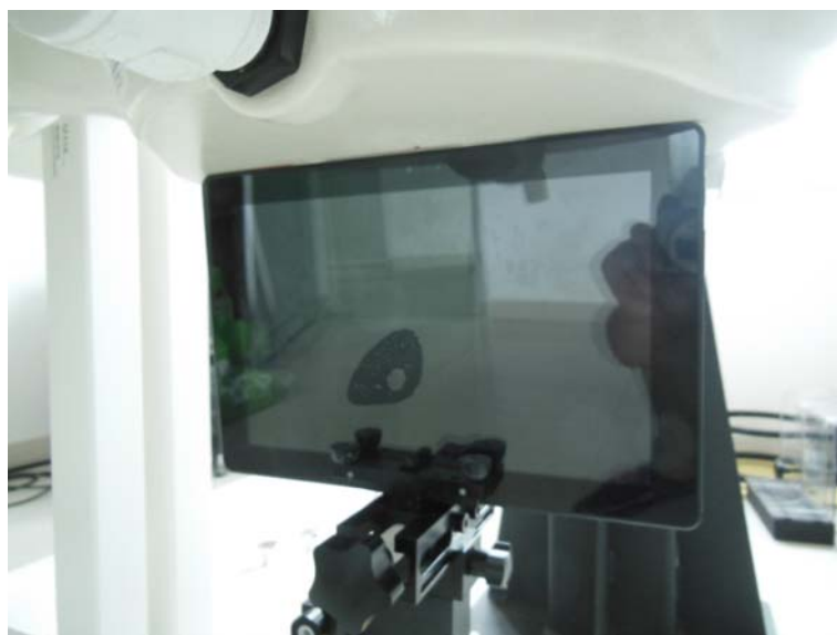
0mm Body-worn Top Side Setup Photo
