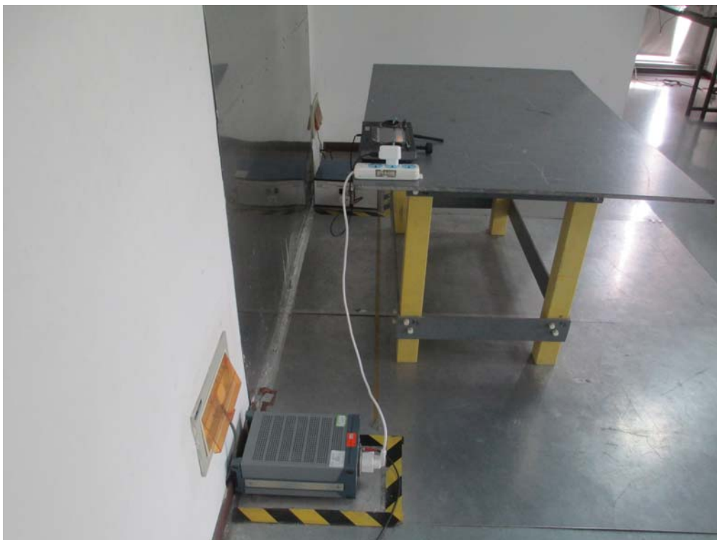
Conducted Emissions Test Setup – Side View
