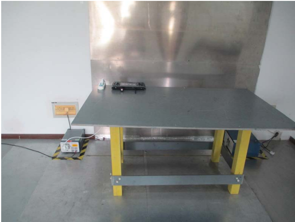
Conducted Emissions Test Setup – Front View
