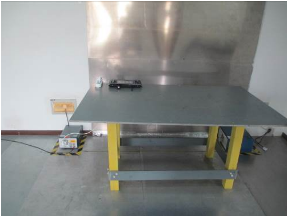
Conducted Emissions Test Setup – Front View
