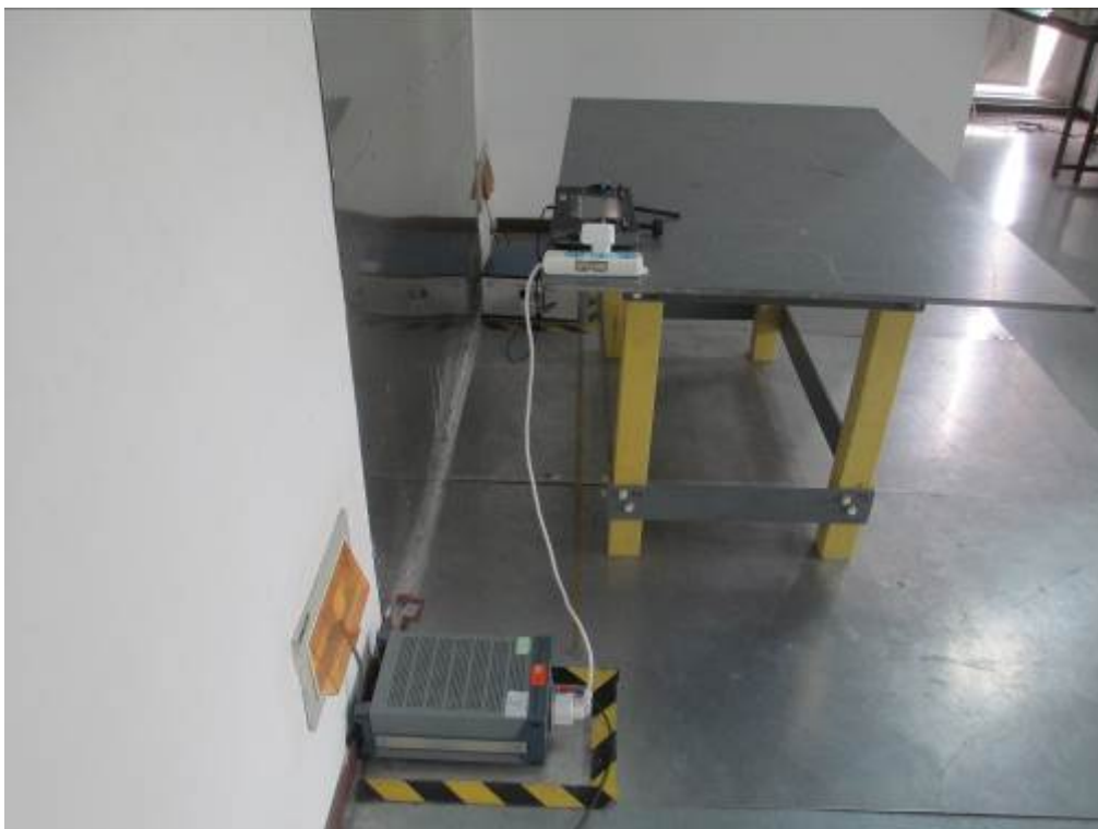
Conducted Emissions Test Setup – Side View
