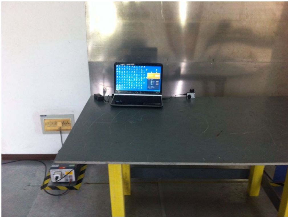
Conducted Emissions Test Setup Front View
