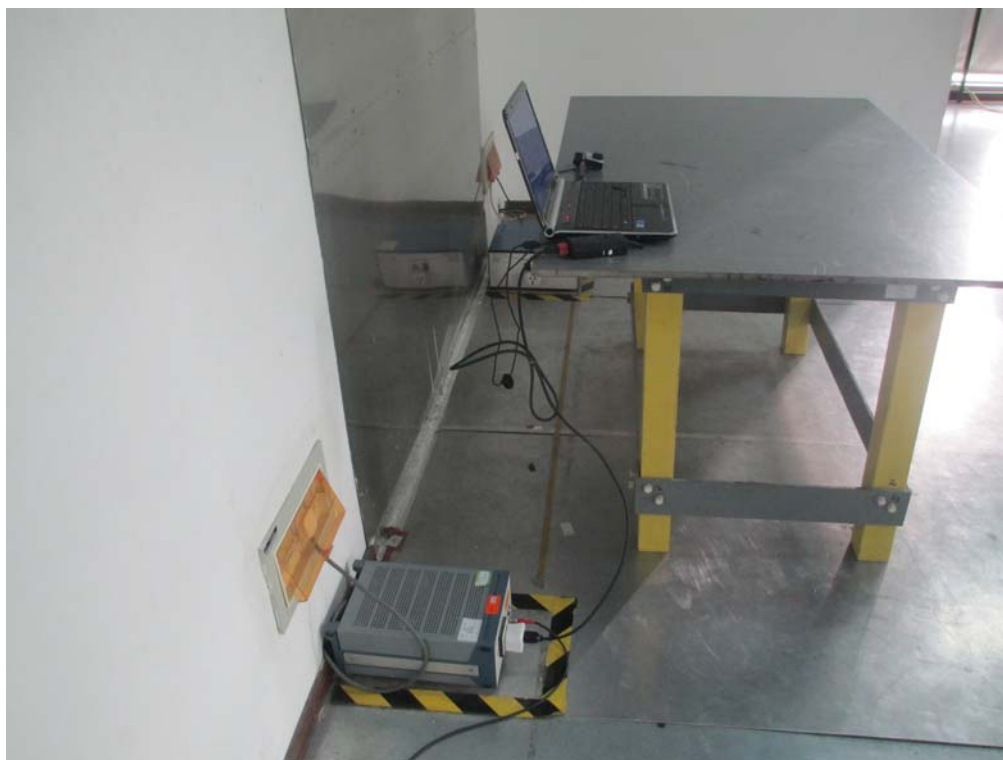
Conducted Emissions Test Setup Side View
