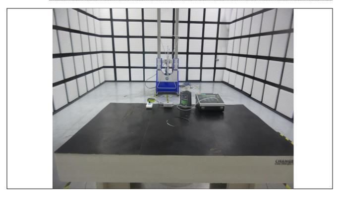
Radiated Emission Test (1000MHz-18000MHz)
