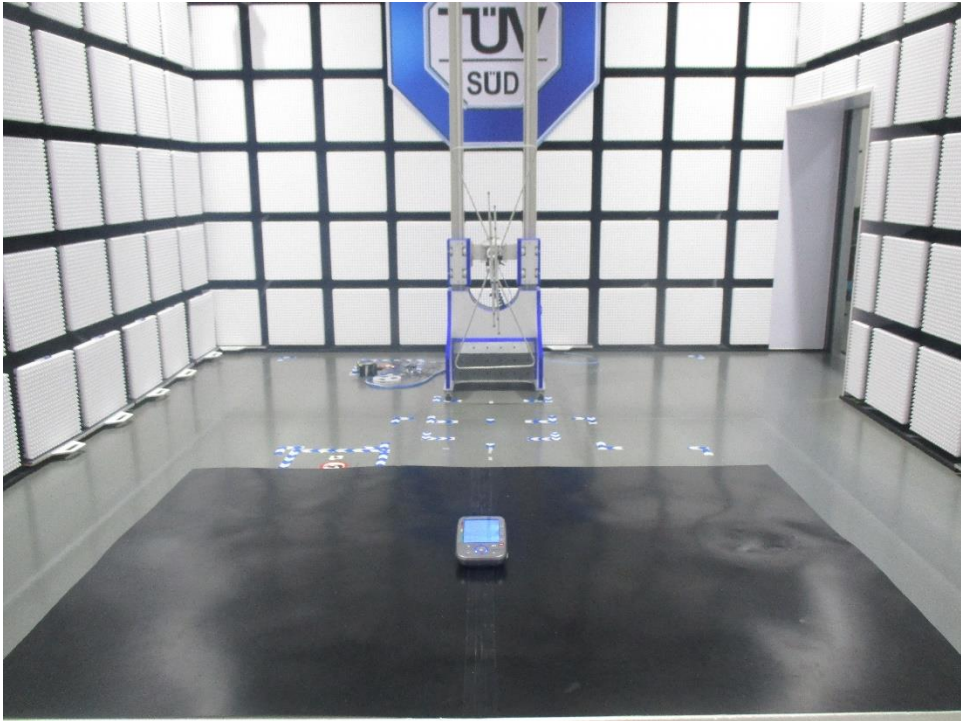
Radiated Emission test of 30MHz-1GHz
