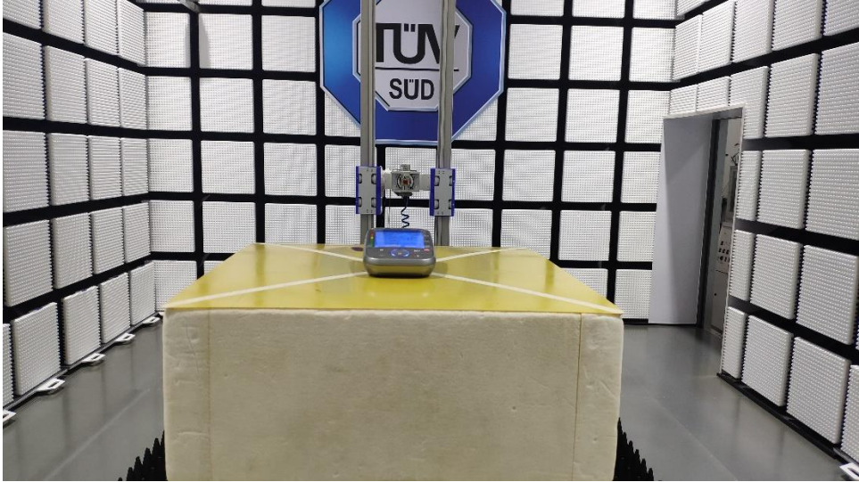
Radiated Emission test 18-25GHz
