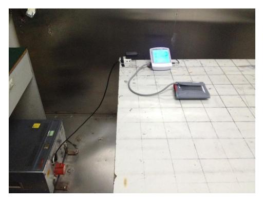
Spurious radiated emission (30MHz-1000MHz)
