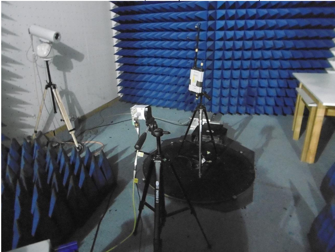
Anechoic chamber (Test setup for 18 GHz – 40 GHz)
