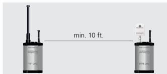
▶ Always keep a minimum distance of 10 feet between the TX and each RX (with mounted 6 dBi antenna and transmission power at -3 dB).
