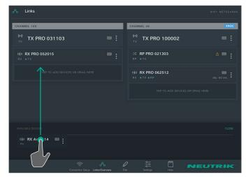
➤ Add an available device to a transmission path: Under Available Devices, use drag&drop to add the device to the transmission path.
