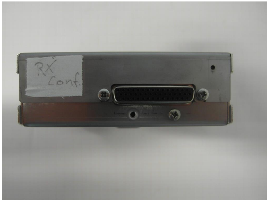
Photo 4 (power supply housing):
