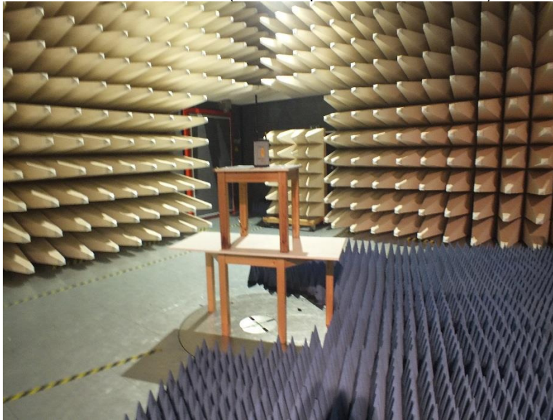
Anechoic chamber (Test setup for 1 GHz – 40 GHz)
