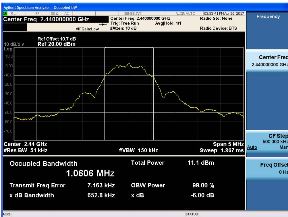
99% Bandwidth plot (Mid-CH 19)
