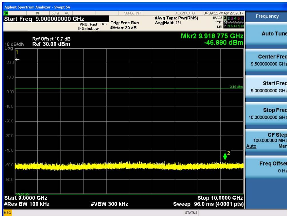
**9.6.2 RADIATED SPURIOUS EMISSIONS****LIMIT : §15.247(d), §15.205, §15.209 / RSS-GEN(Issue 4) Section 8.9**
