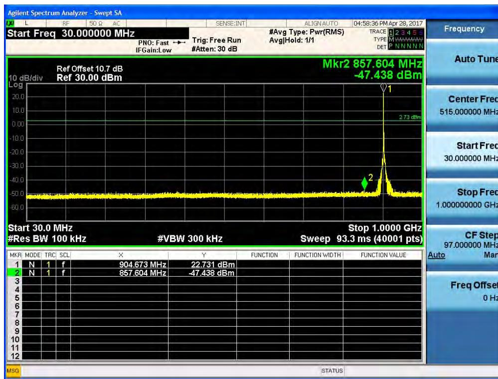
Test Plots (DBPSK)- 1 GHz – 3 GHz
