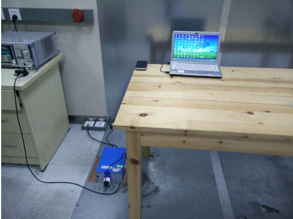
Radiated Spurious Emissions From 30MHz-1000MHz
