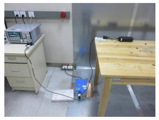
FCC RADIATED EMISSION TEST SETUP
