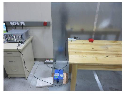
FCC RADIATED EMISSION TEST SETUP
