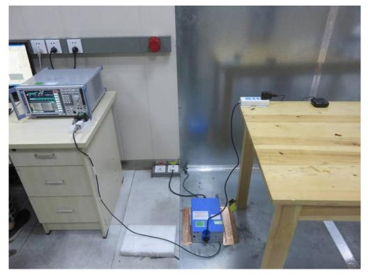
FCC RADIATED EMISSION TEST SETUP
