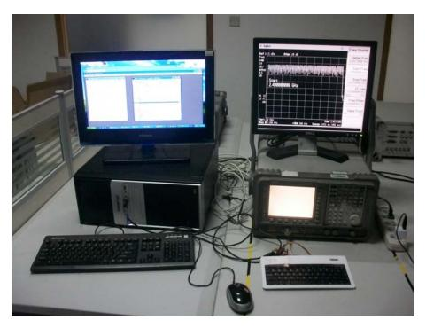
SPURIOUS EMISSION TEST SETUP
