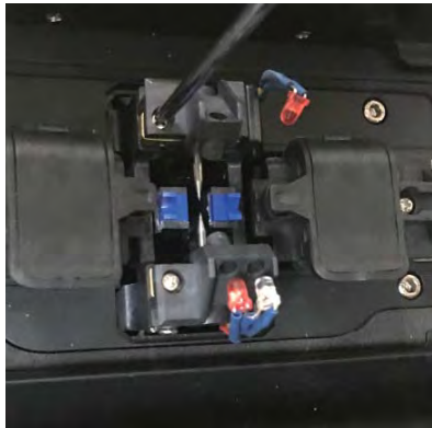
5. Screw out the screws with a screwdriver
