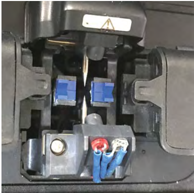
13. Replace the other electrode by the same way
