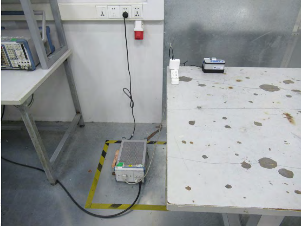
Photo of Power Line Conducted Emission Test
