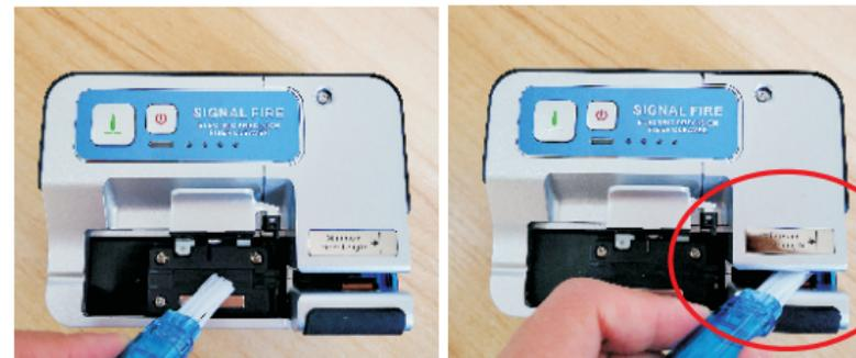
When there are waste fibers or debris on the left and right splints, the fibers cannot be clamped or the fibers cannot be cut.
