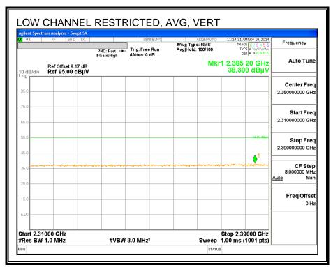
Corrected Value = Marker reading + Duty Cycle Factor Final Corrected Average Value: 39.399dBuV + 3.72 = 43.119dBuV
