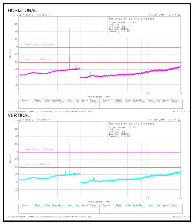
Note: Emission was scanned up to 26GHz; No emissions were detected above the noise floor which was at least 20dB below the specification limit.
