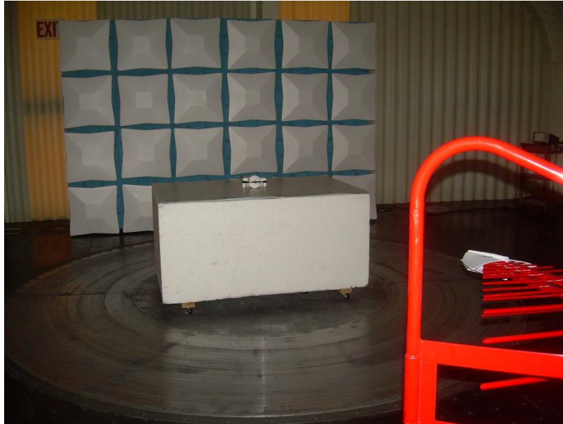
Photograph 1: Front View Radiated Emissions – 30 to 1000 MHz
