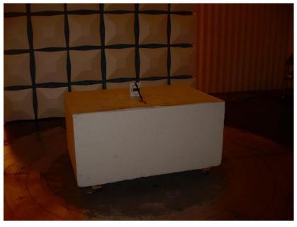
Photograph 1: Front View Radiated Emissions Worst-Case Configuration – Below 1000 MHz
