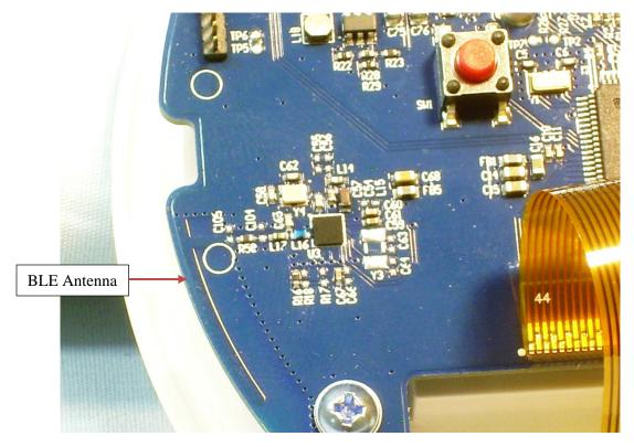
Photograph 16: View of the PCB Antenna for the BLE Transceiver
