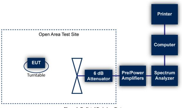
Figure 1: Radiated Emissions Test
