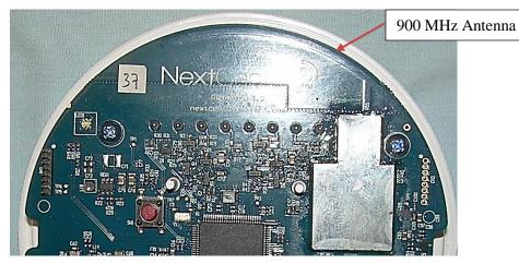
Photograph 15: View of the PCB Antenna for the 900 MHz Transceiver
