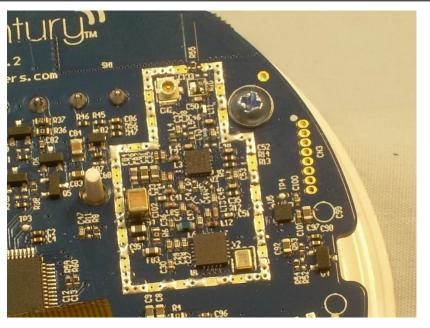
Photograph 13: View of the Circuitry Under the RF Shield
