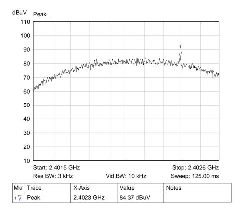
Graph 9: Lowest Channel 3 kHz PSD Plot
