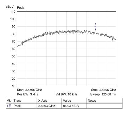
Graph 11: Highest Channel Output 3 kHz PSD Plot
