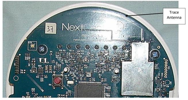
Photograph 4 – 900MHz Trace Antenna
