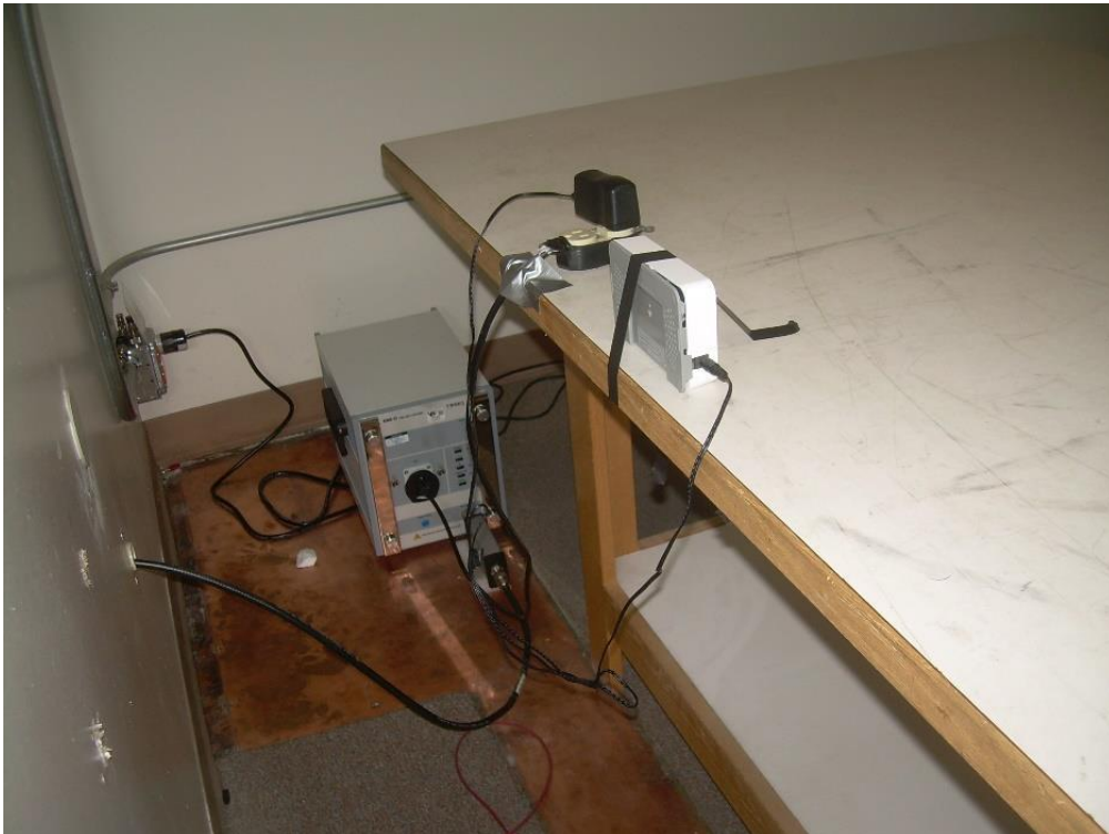
Photograph 6: Back View Conducted Emissions Worst-Case Configuration
