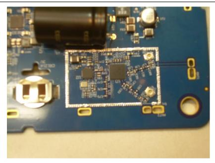
Photograph 15: View of the Circuitry Under the 900 MHz Transceiver RF Shield
