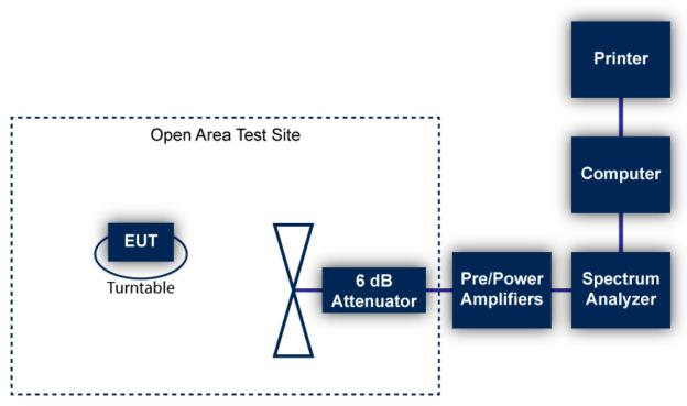
Figure 3: Radiated Emissions Test
