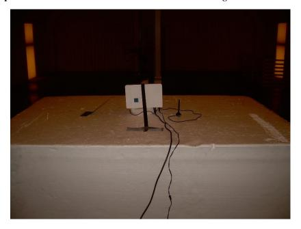
Photograph 4: Back View Radiated Emissions Worst-Case Configuration – Above 1000 MHz
