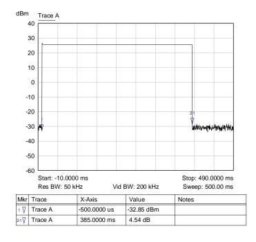
**Graph 7: Timing Plot Showing Duration of Channel On Time**
