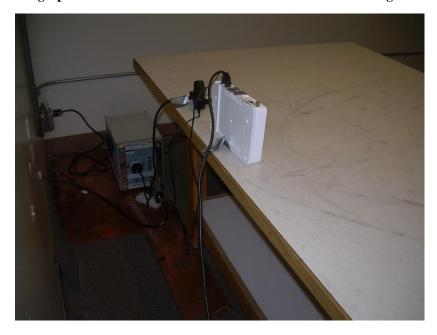
Photograph 6: Back View Conducted Emissions Worst-Case Configuration
