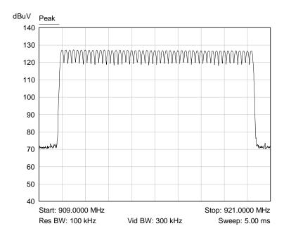
Graph 13: Antenna 2 - Plot Showing All Channels Operate Within the Authorized Frequency Band
