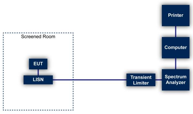
Figure 1: Conducted Emissions Test
