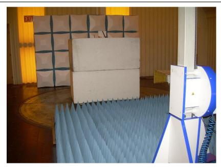
Photograph 3: Front View Radiated Emissions Worst-Case Configuration – Above 1000 MHz
