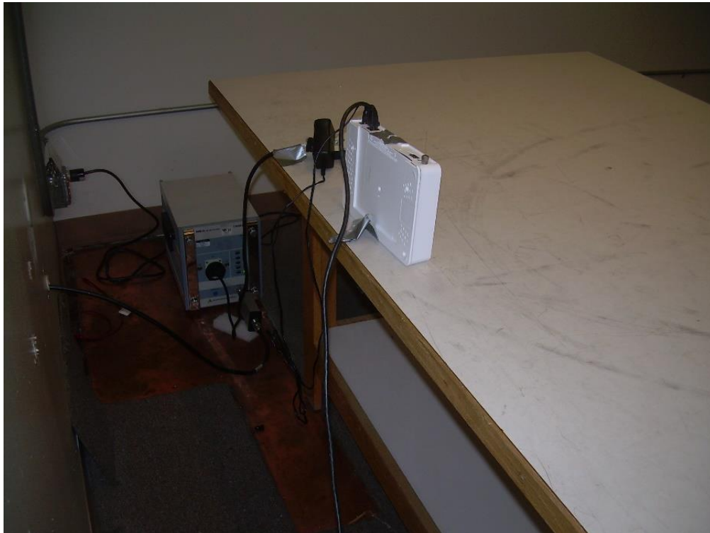
Photograph 6: Back View Conducted Emissions Worst Case Configuration
