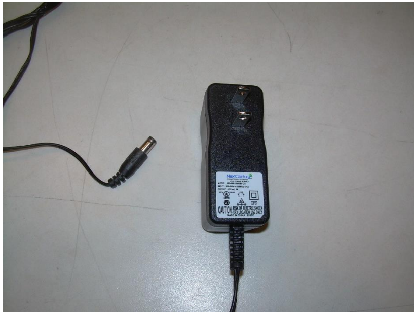
Photograph 12: View of the Power Supply
