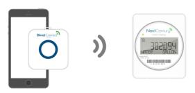
The DC301 wireless programmer facilitates configuration of NextCentury 301+ devices such as the RR301 Remote Reader.
