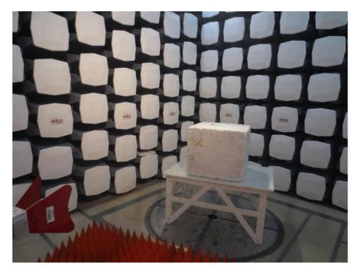
1.2. EUT Setup at 3 Meters (Above 1GHz)
