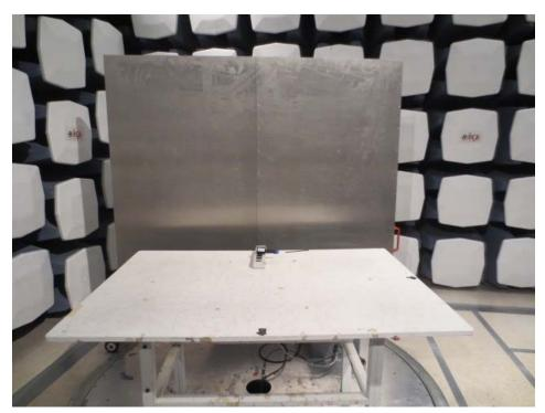
**15.2** Conducted Emissions - Side View with AC/DC Adapter
