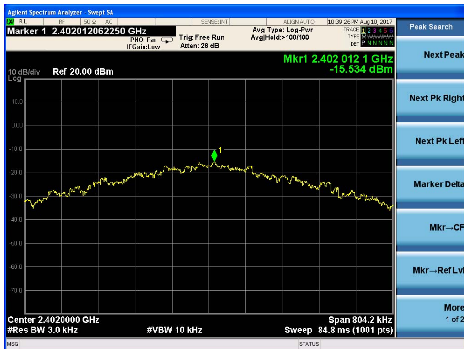
Power spectral density plot on channel 00
