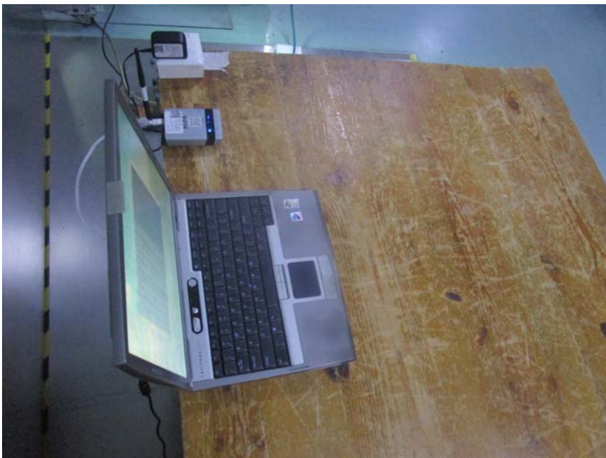
Conducted Emissions– Side View(AC/DC Adapter)
