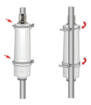
How to install the antenna
