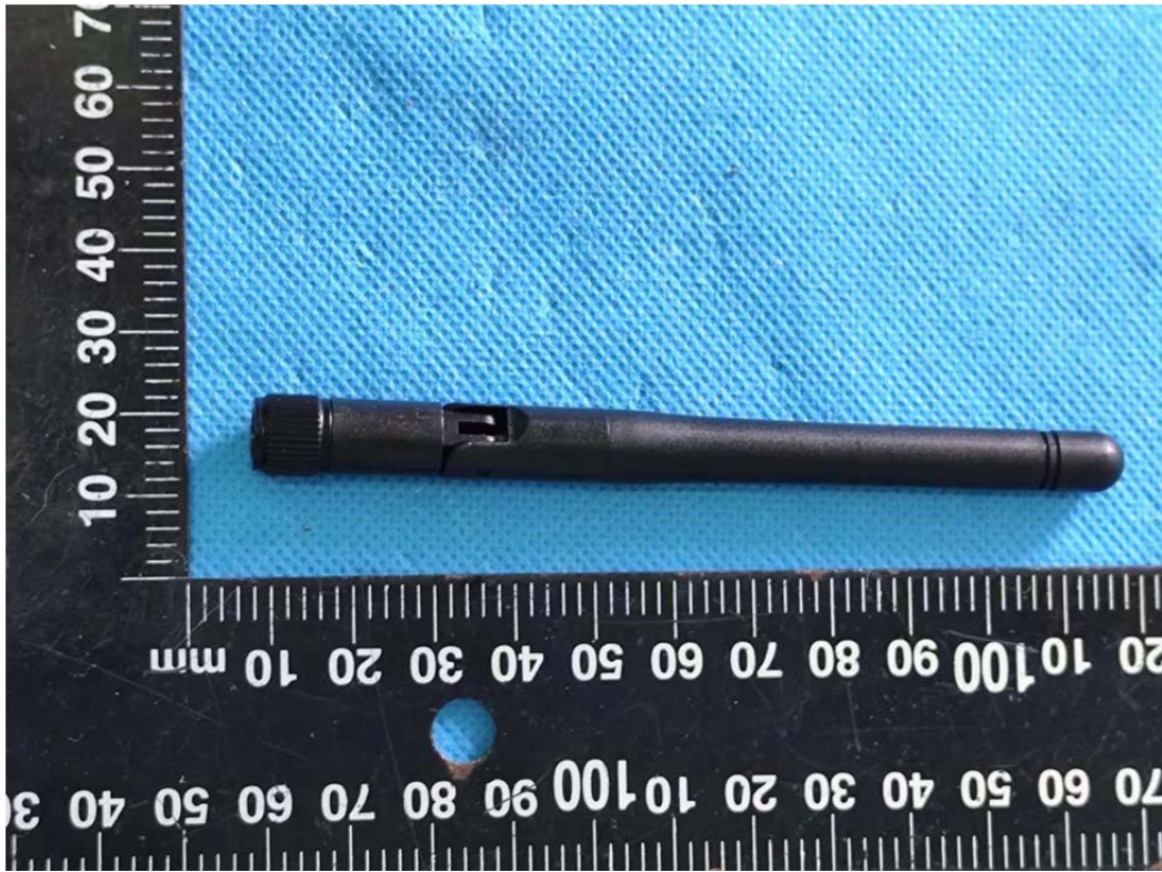
Wi-Fi Chain 0 Antenna
