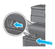
2 Pull the Punch Kit Release Lever [FS2] in the arrow direction, and open the Punch Kit.
