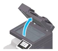
2 Wipe stains off the Slit Scan Glass using a dry, clean cloth.
