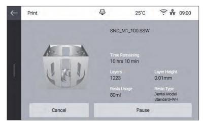
If chamber temperature is lower than the target, heater will heat up the inside of the chamber. When chamber temperature reaches the target, printing starts.
