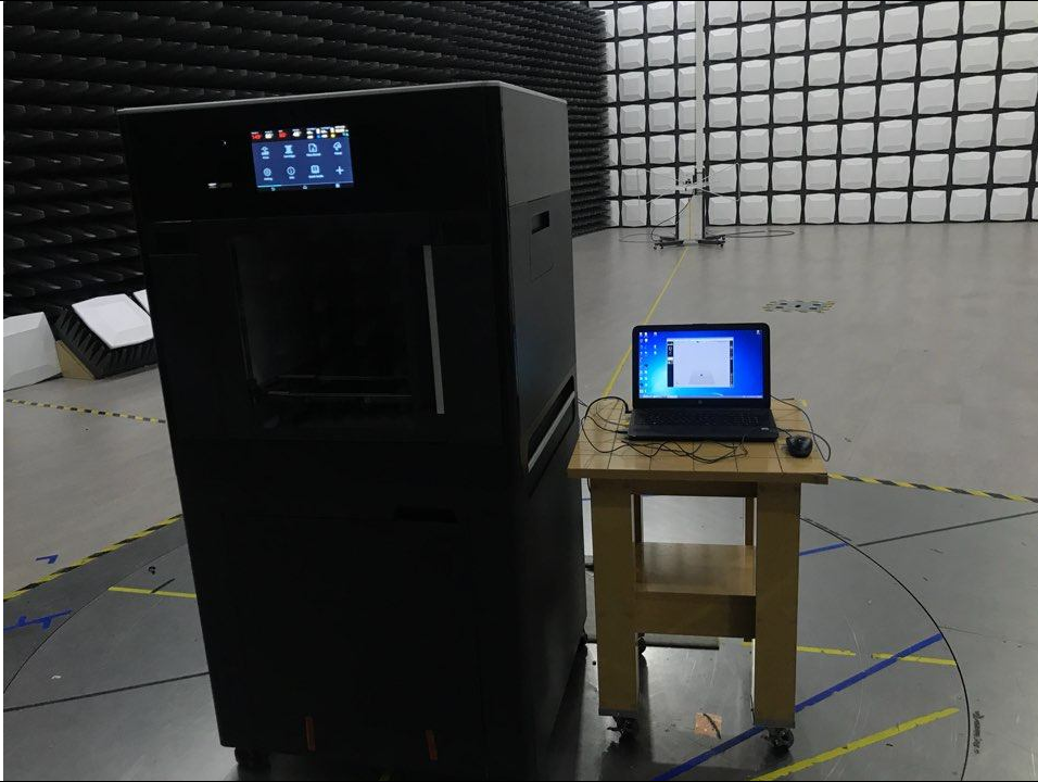
Mode #1 ~ #5 _ Test Setup for 30 MHz ~ 1 GHz
