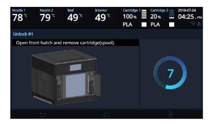
4 After 10 seconds printer will automatically change to [LOCK] state and [UNLOCK] appears.
