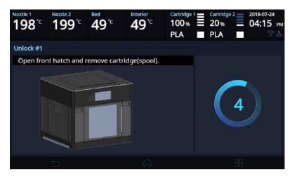
2 After 10 seconds printer will automatically change to [LOCK] state and [UNLOCK] appears.
