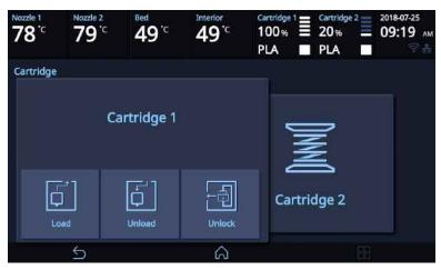
When [OK] is pressed at the cartridge load confirming message, cartridge load will automatically proceed. The filament reaches to the nozzle and it is heated up to the specified temperature. Then the filament is inserted into the heated nozzle. After the process has finished, screen will automatically return to the [HOME] screen.
