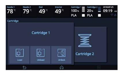
For 10 seconds **[LOCK]** state is deactivated and the user can detach cartridge from printer.
