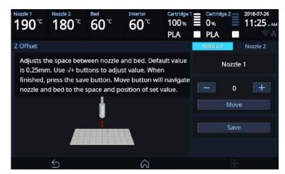
4 Use the [Move] and [Save] buttons to adjust the gap and to save the setting.
