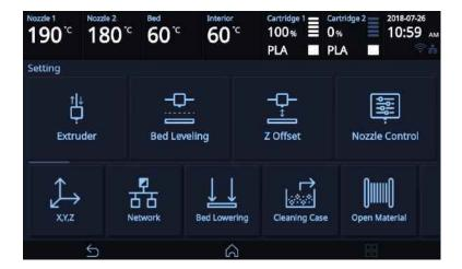
3 To Control [Extruder], Nozzle temperature needs to be raised.
