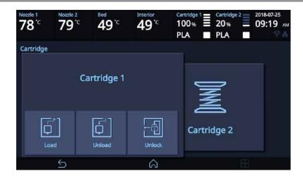
When **[OK]** is pressed at the cartridge unload confirming message, cartridge unloading will automatically proceed. To remove filament, the nozzle is heated up to the specified temperature and the filament unload starts.
