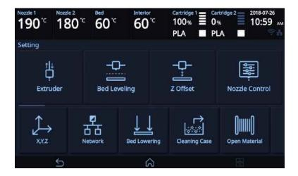
3 Select the nozzle that you will use to adjust the gap. Default value is 0.25mm, Use [+], [-] buttons to move in 0.05 mm unit.
