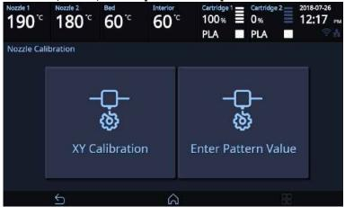
Press the [Yes] button to access the XY Calibration printing screen.
