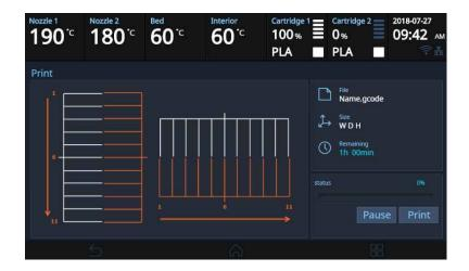
6 After printing the XY calibration pattern, enter the number of the line that is most linear among those printed with nozzles 1 and 2, and then press the [Save] button. Select the most linear line (No.1 starts from the top for horizontal lines and from the left for vertical lines)
