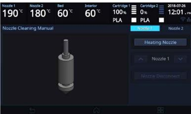
Press the [Heating nozzle], Set the temperature and start Heating Nozzle.
