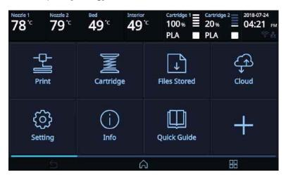
2 Press the [Nozzle Control], [Nozzle cleaning Manual] button to access nozzle cleaning settings. Select the nozzle that you want to clean.
