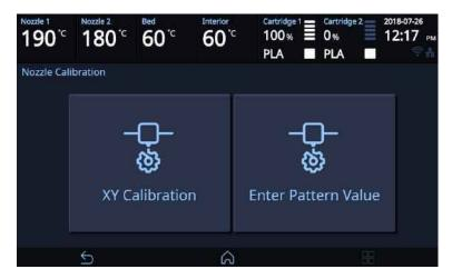
4 Enter the values for the horizontal and vertical lines. And press [Save] button.
