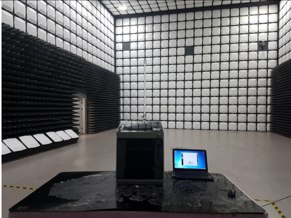
Mode #1 ~ #5 Test Setup for 30 MHz ~ 1 GHz
