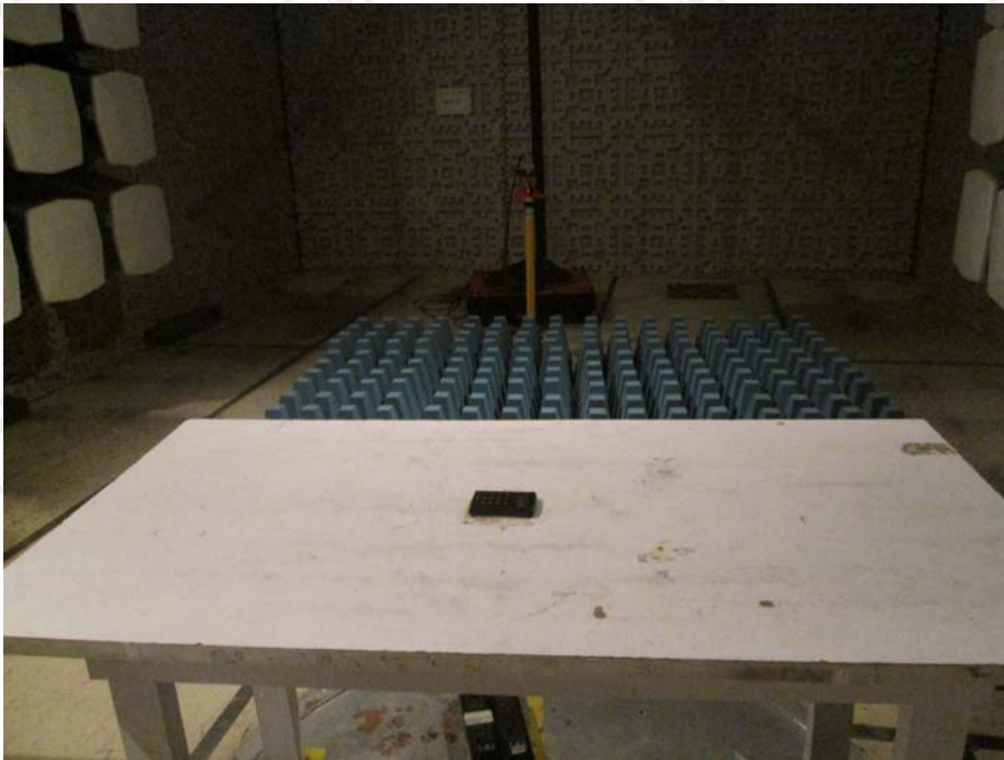
TEST SETUP OF RADIATED EMISSION (above 1GHz)
