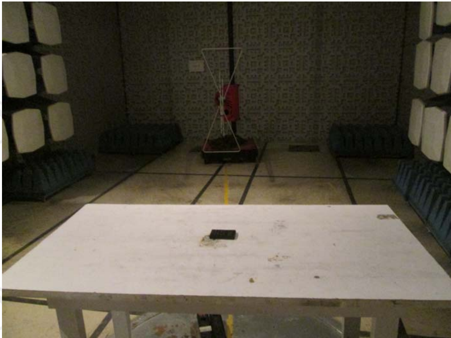
TEST SETUP OF RADIATED EMISSION (30MHz-1GHz)
