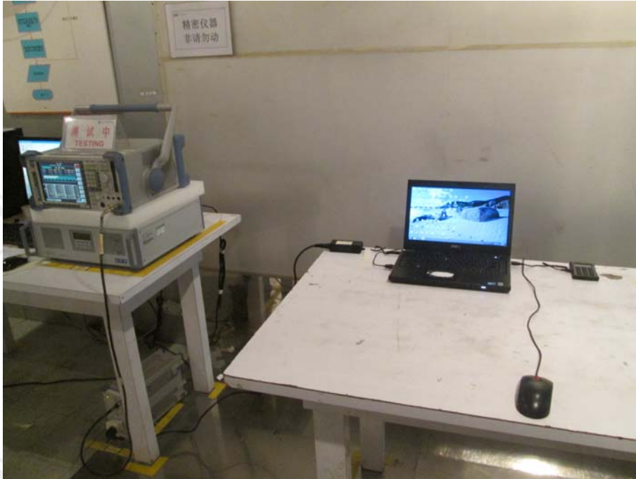
CONDUCTED EMISSION TEST SETUP
