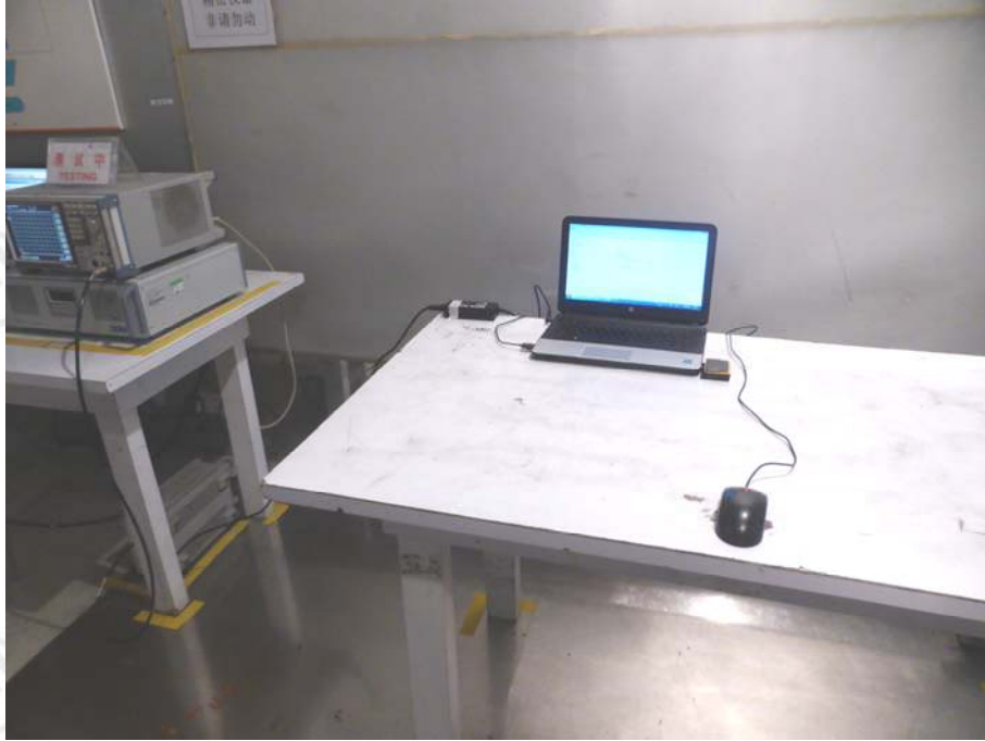
TEST SETUP OF CONDUCTED EMISSION
