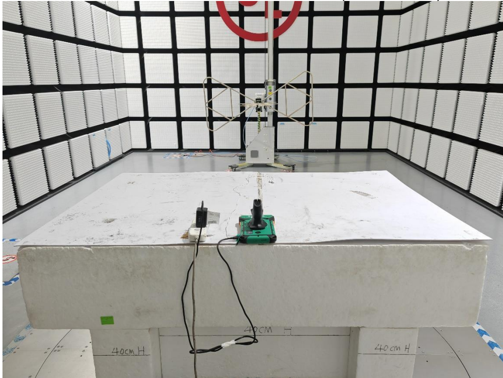
RADIATED RF MEASUREMENT SETUP (30MHz~1GHz)
