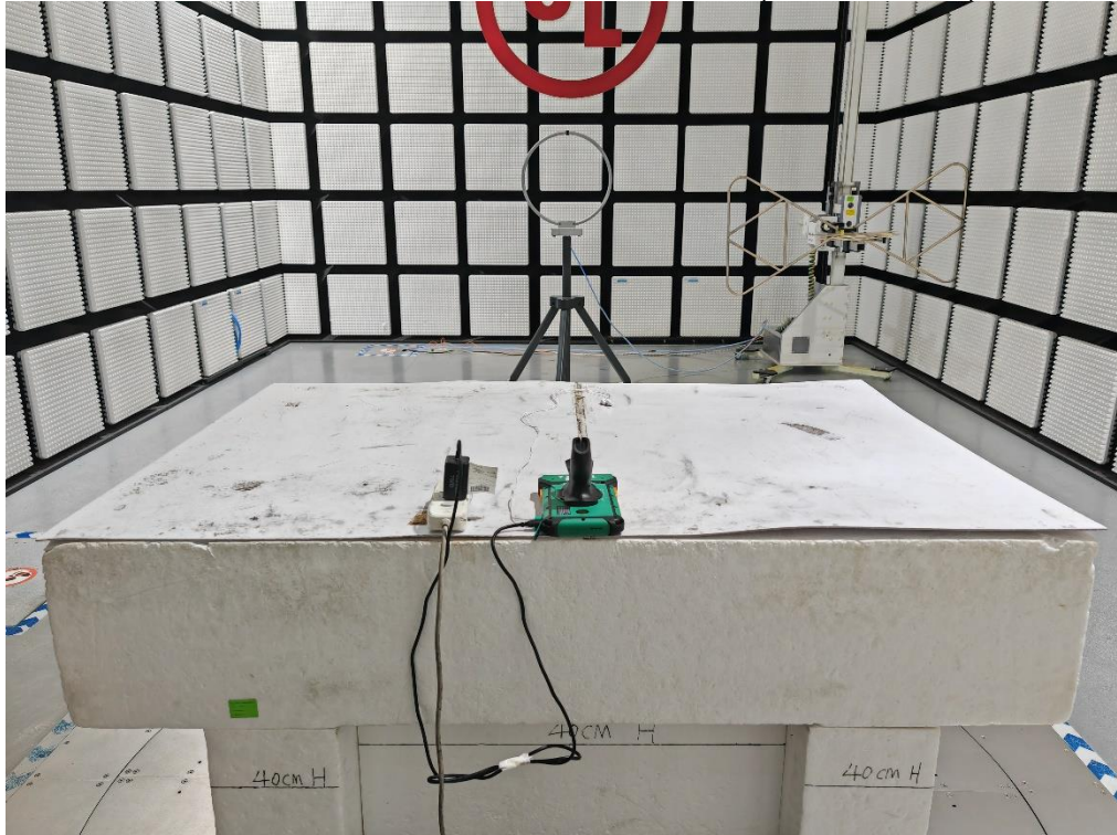
RADIATED RF MEASUREMENT SETUP (Below 30MHz)
